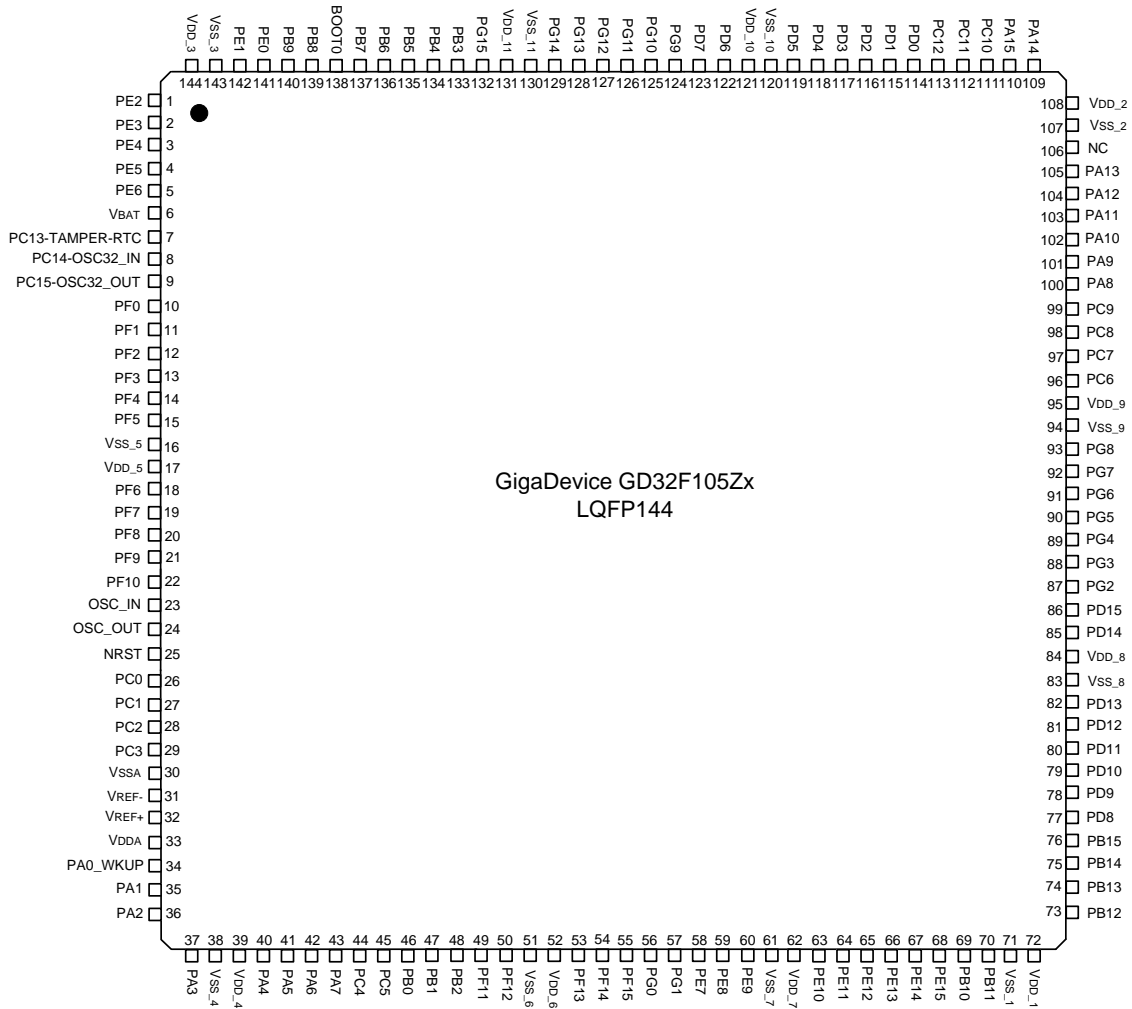
Figure 2. GD32F105Zx LQFP144 pinouts
